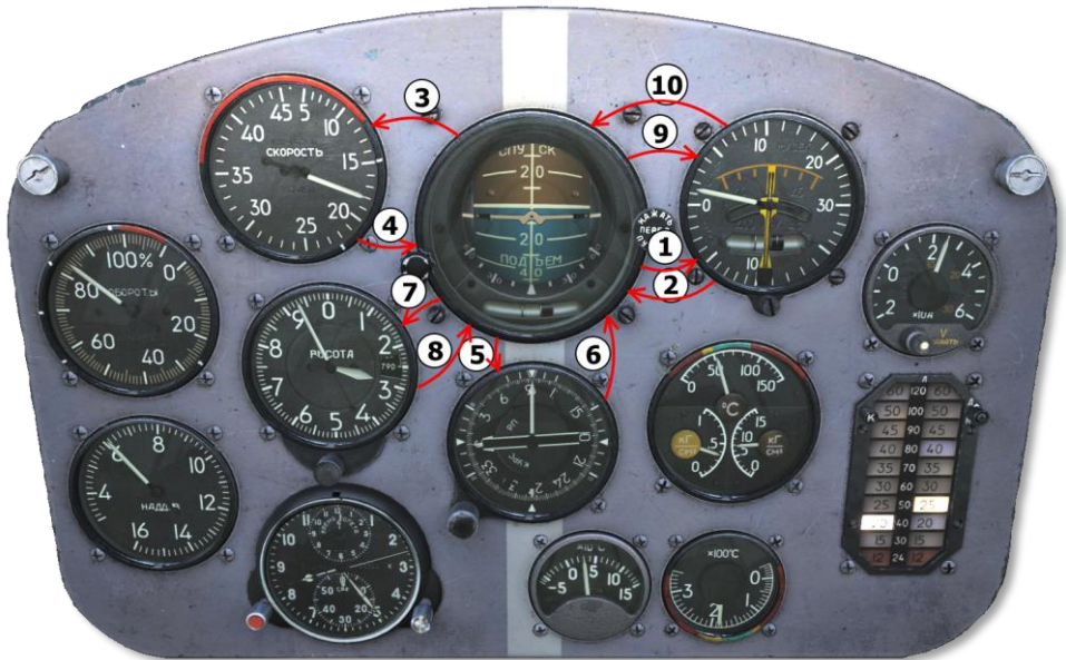
Figure 62. Instrument checking rotation for level flight.
