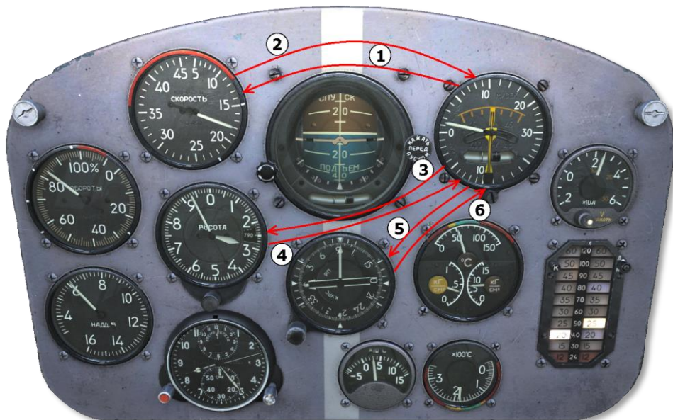
Figure 68. Instrument checking rotation during flight using the DA-30.
