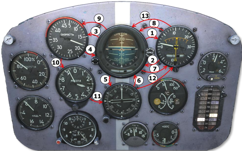
Figure 63. Instrument checking rotation during climbing.
