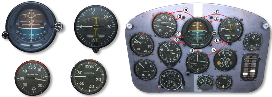
Figure 64. Instrument checking rotation during gliding.
